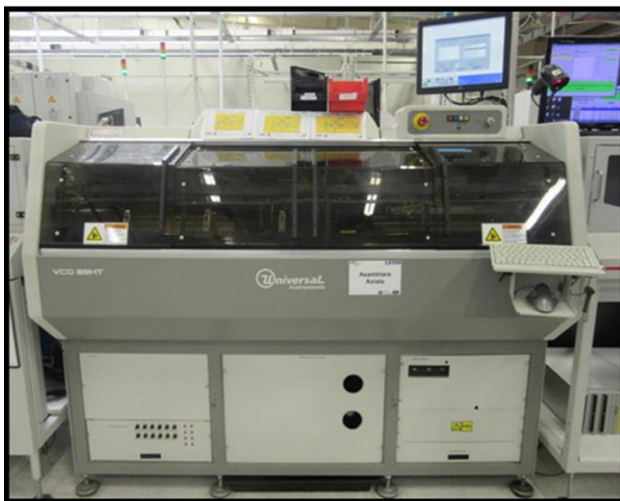
Fig. 7. The axial machine
