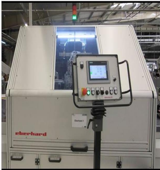
Fig. 10. Eberhard - the machine used to insert the pins
