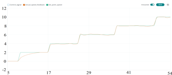
Fig. 44. Setpoint and feedback went up gradually from 0-2-4-6-8-10 reps/min
