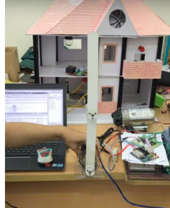
Fig. 21. Pendubot is at TOP position under LQR controller.
