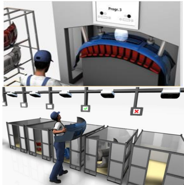
Fig. 3. The worker places the bumper in the transport box indicated by the system [9]
