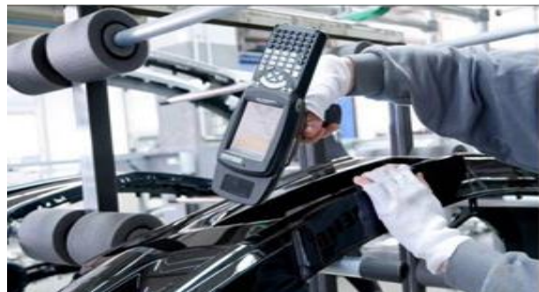
Fig. 4. Bumpers identified with RFID tags throughout the production and logistics process. [4]
