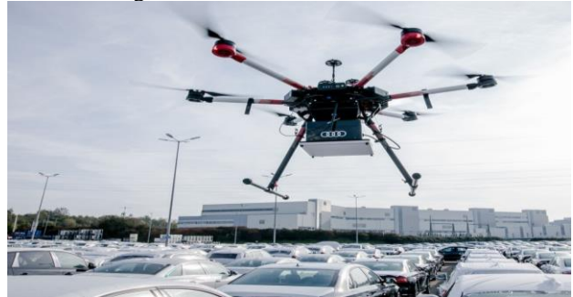
Fig.12. Inspection of the car park with the help of the Hexacopter drone [14]
