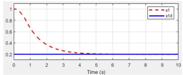
Fig. 11. Comparison between angle of link 1 and reference trajectory (rad)
