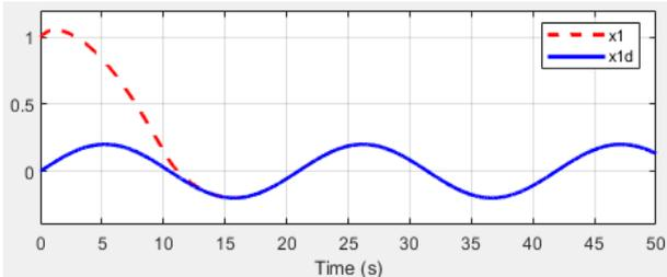
Fig. 7. Comparison between angle of link 1 and reference trajectory (rad)
