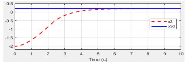
Fig. 12. Comparison between angle of link 2 and reference trajectory (rad)
