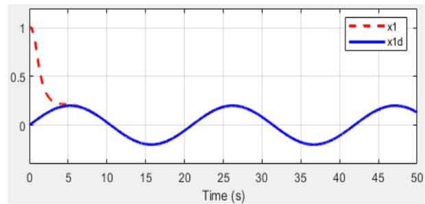
Fig. 3. Comparison between angle of link 1 and reference trajectory (rad)
