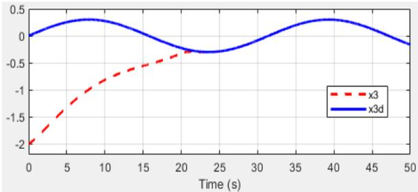
Fig. 8. Comparison between angle of link 2 and reference trajectory (rad)
