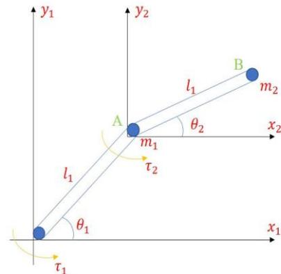
**Fig. 1.** Mathematical model of a two-linked robot arm.
