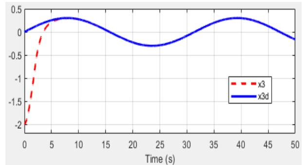
Fig. 4. Comparison between angle of link 2 and reference trajectory (rad)
