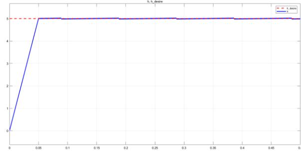
Fig. 14. The output response of the system with  $k_{SMC} = 100$  (red: setpoint; blue: height of water in tank)
