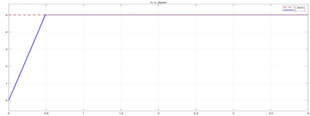
**Fig. 10.** The output response of the system with  $k_{SMC} = 10$  (red: setpoint; blue: height of water in tank)
