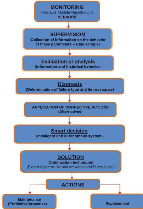
Fig. 19. Flowchart of intelligent monitoring and supervision system. [5]
