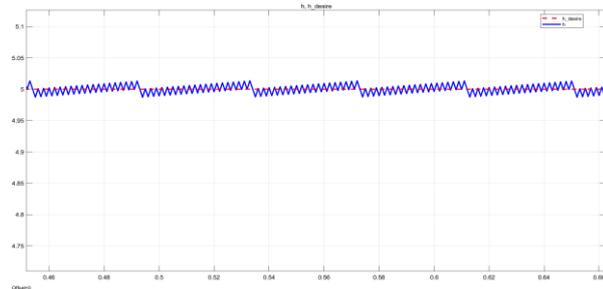
Fig. 13. Zoom-in output response of the system with  $k_{SMC} = 40$  (red: setpoint; blue: height of water in tank)
