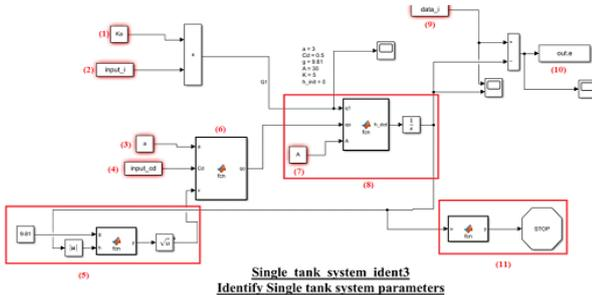
Fig. 6 Matlab program identify parameters of single water tank system
