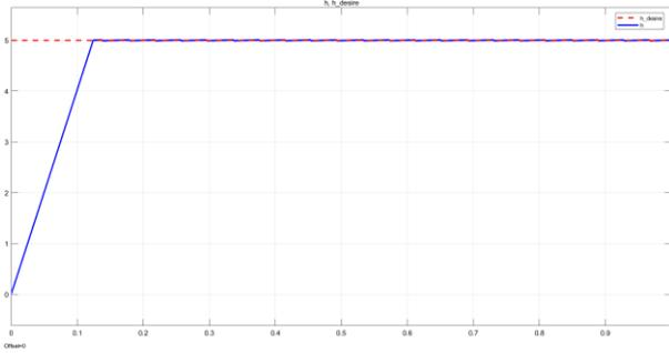
Fig. 12. The output response of the system with  $k_{SMC} = 40$  (red: setpoint; blue: height of water in tank)
