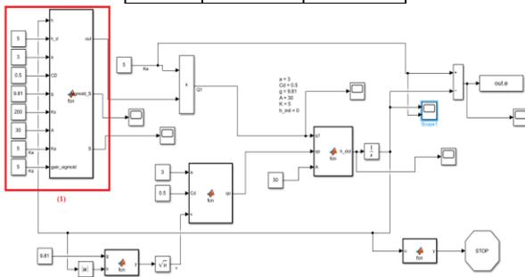
**Fig. 9.** Simulation of SMC for single water tank
