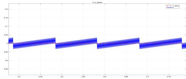
Fig. 15. Zoom-in output response of the system with  $k_{SMC} = 100$  (red: setpoint; blue: height of water in tank)
