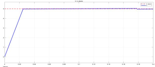
Fig. 16. The output response of the system with  $k_{SMC} = 200$  (red: setpoint; blue: height of water in tank)
