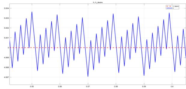
**Fig. 11.** Zoom-in output response of the system with  $k_{SMC} = 10$  (red: setpoint; blue: height of water in tank)
