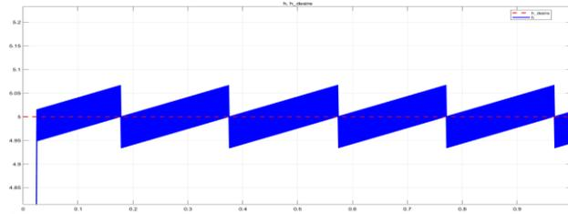
Fig. 17. Zoom-in output response of the system with  $k_{SMC} = 200$  (red: setpoint; blue: height of water in tank)
