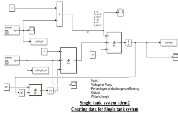
Fig. 5. Simulation program generates sample data for single water tank system
