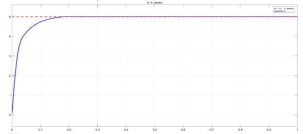
Fig. 18. The output response of the system using FSMC at setpoint  $h_{desire} = 5$  cm (red: setpoint; blue: height of water in tank)
