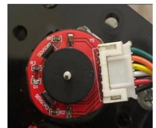
**Fig. 13.** Encoder in back of DC motor GA25-370
