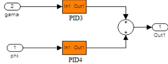
Fig. 4. PID structure that controls angle of tower and rotational angle of load
