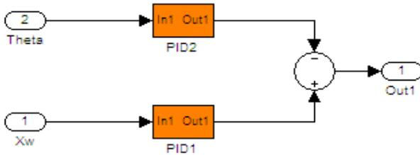
Fig. 3. PID structure that controls position of trolley and dimensional angle of load
