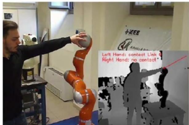
**Fig. 8.** On-line estimation of contact forces [11].
