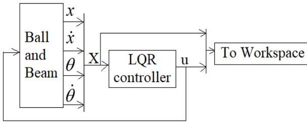
Fig. 2. LQR control structure for B&B
