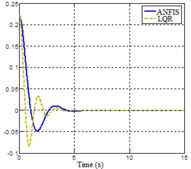
Fig. 9. Position of ball (m)
