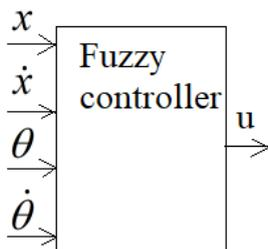
Fig. 3. Structure of fuzzy controller from ANFIS toolbox
