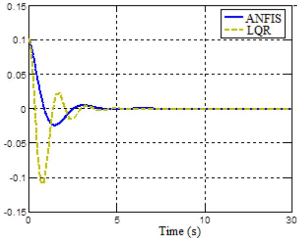
Fig. 7. Position of ball (m)
