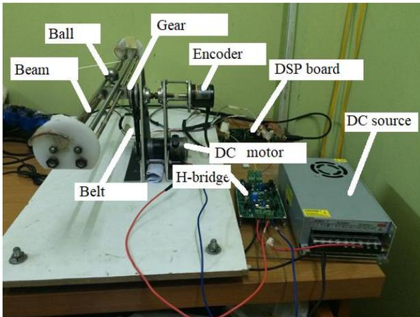
Fig. 11. Hardware platform of B&B in HCMUTE
